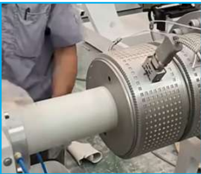
Fig: Pipe is cut and socket made and printed by the machine
