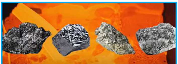
Fig: Addition of carbon, silicon, manganese and magnesium to molten iron scrap to improve its strength and flexibility
