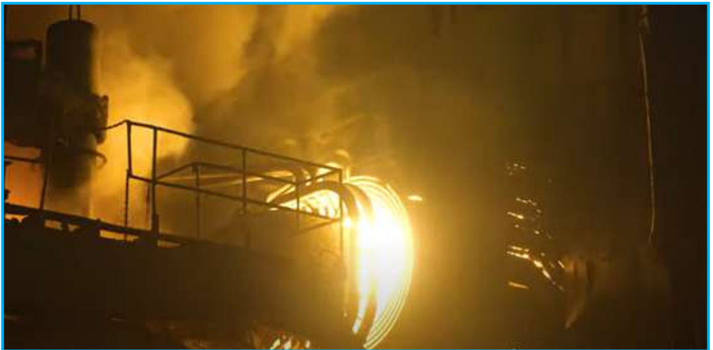
Fig: Molten Iron is inserted in ventilated chamber container exhaust fans activated to manage fumes and draws out the smoke produced during melting process and as the metal melts impurities within the molten rise to the surface and form a layer
