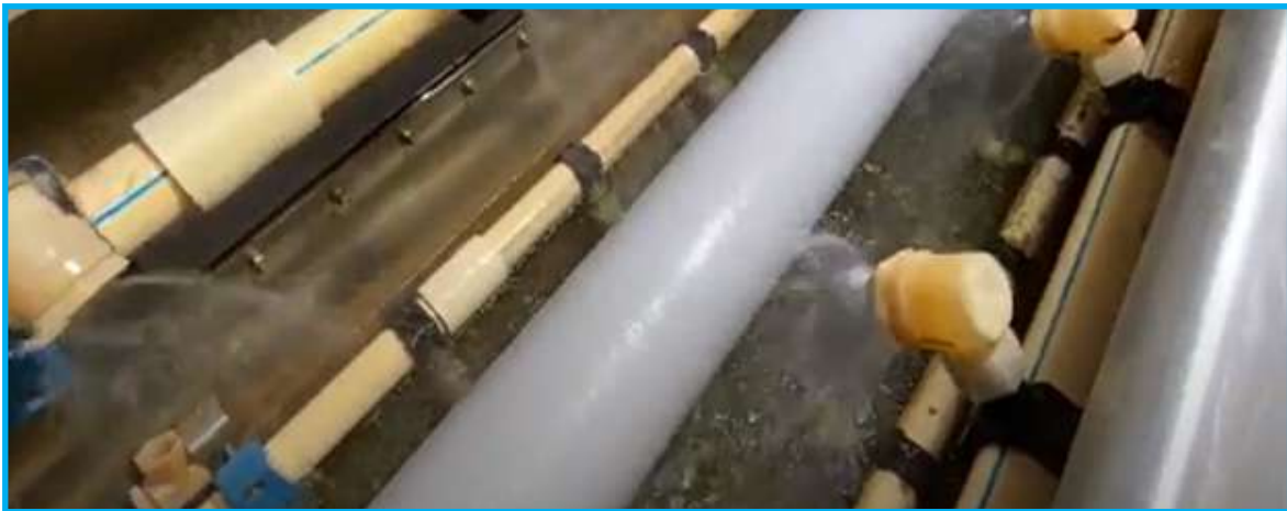
Fig: Pipe is cooled here by spraying water
