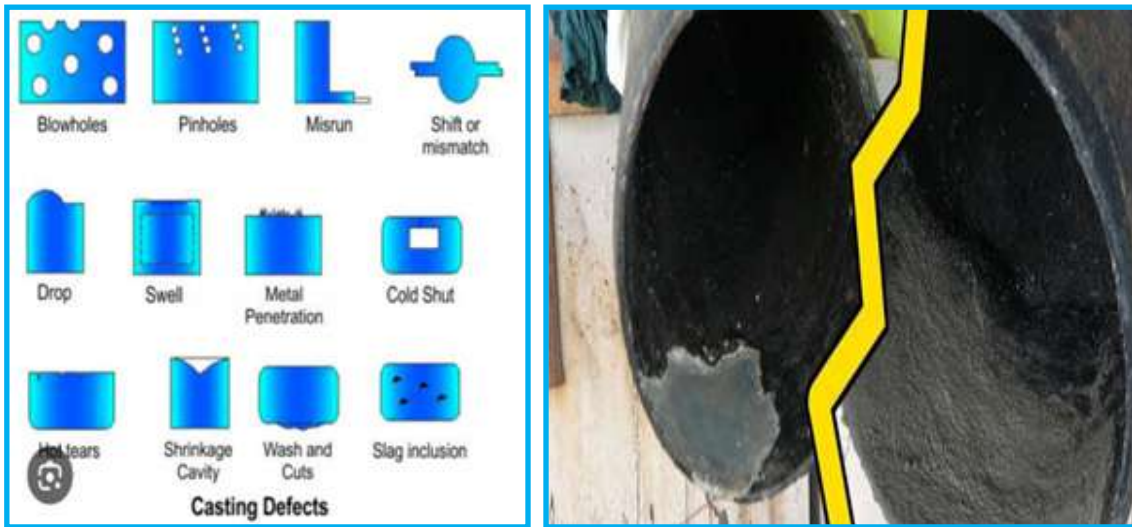
Fig: Casting and Cement lining defect of DI Pipe
