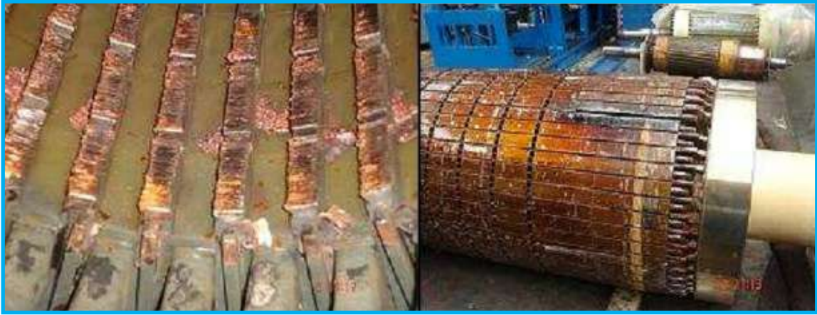
Fig: Damage of Stator and Rotor of a Pump
