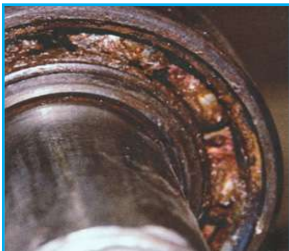
Fig: Damage of Bearing of a Pump
