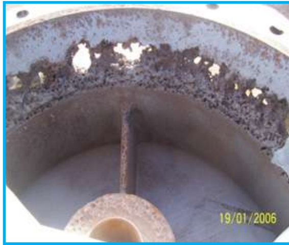
Damage of Pump casing of a Centrifugal Pump
