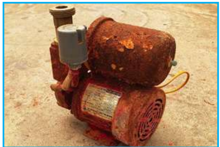
Fig: Damage of Housing assembly of a Centrifugal Motor
