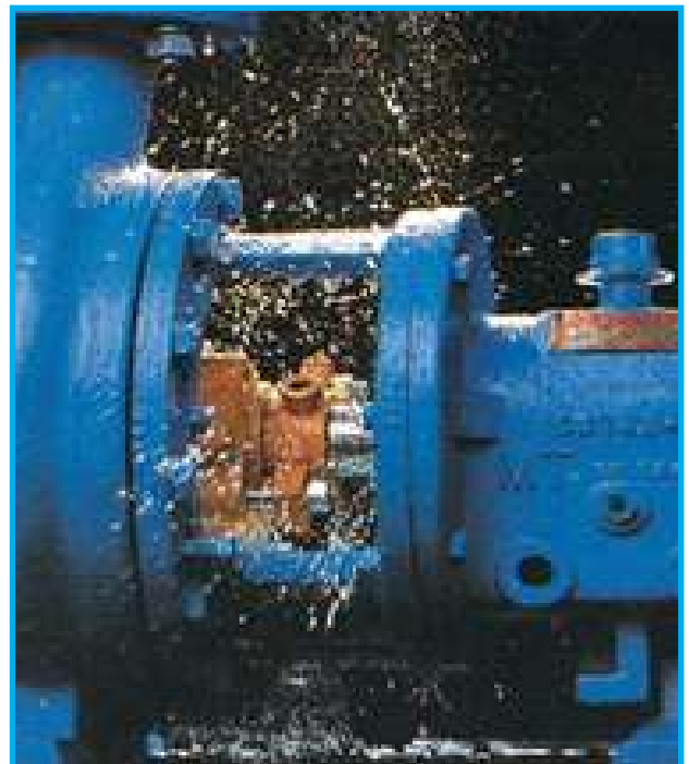
Fig: Damage of Mechanical Seal or Packing of a Pump
