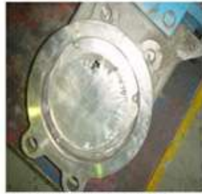
2 : Uni-directional valve with deflection cone subjected to reverse slurry flow
