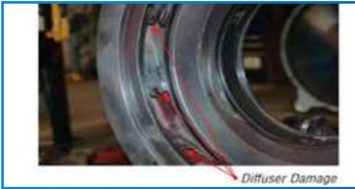
Fig: Damage of guide vane of submersible pump
