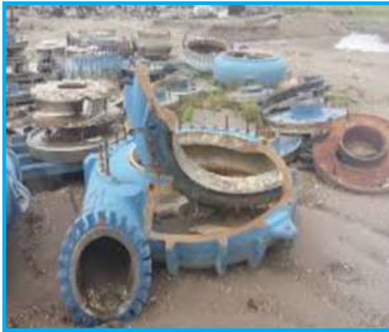
Damage of Pump casing of a Centrifugal Pump
