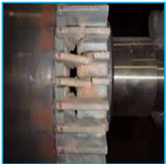
Fig: Damage of Stator and Rotor of a Pump
