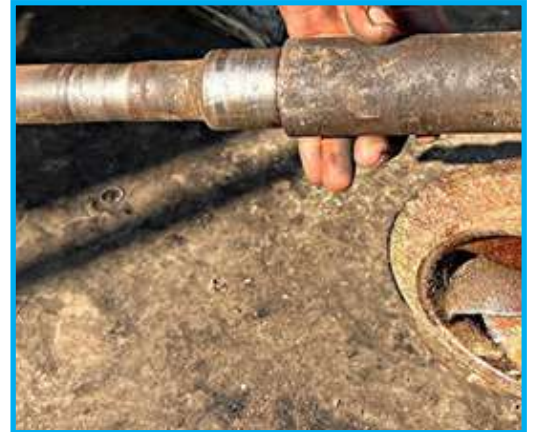
Fig: Damage of Pump shaft of submersible pump
