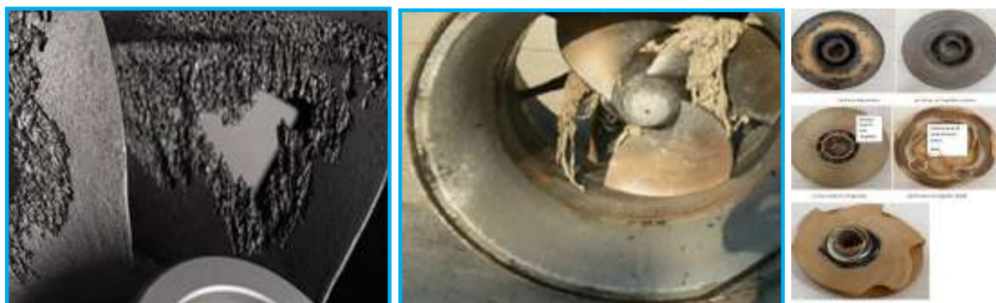
Fig: Damage of impeller of submersible pump
