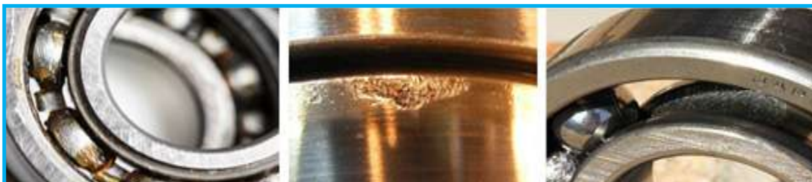
Fig: Damage of Motor Bearing of a Pump
