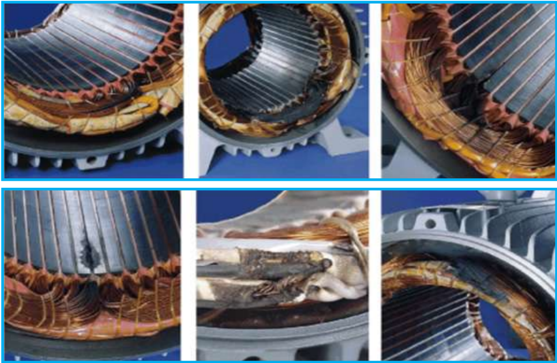
Fig: Damage of Stator and Rotor of a Pump
