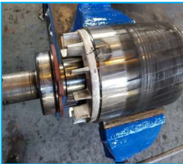
Fig: Damage of Stator and Rotor of a Pump
