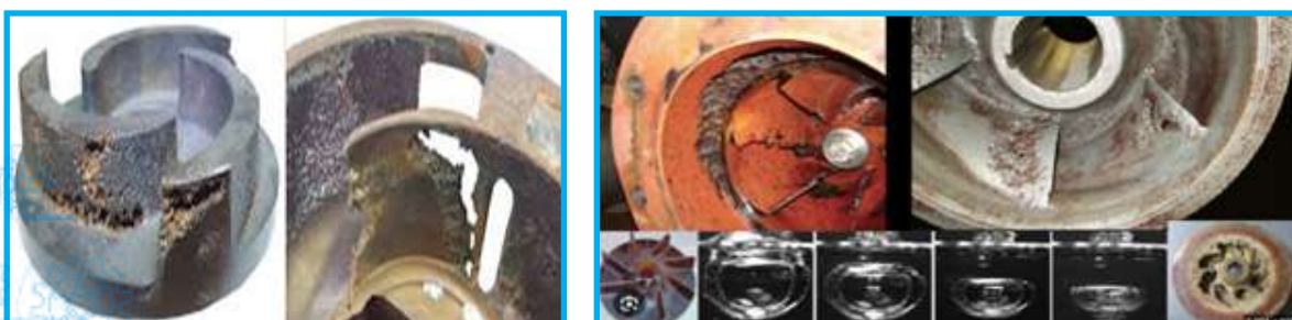
Fig: Damage of Wear Rings of a Pump
