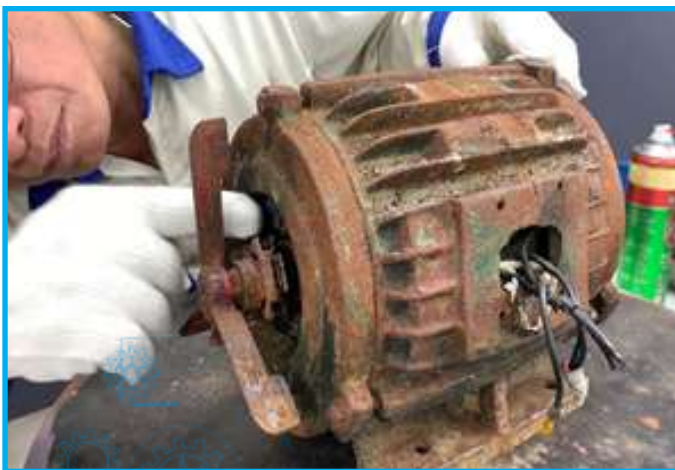
Fig: Damage of Housing assembly of a Centrifugal Motor
