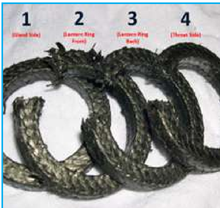
Fig: Damage of Mechanical Seal or Packing of a Pump
