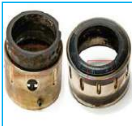
Fig: Repair methods of Mechanical seal of submersible pump
