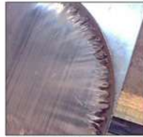
3 : Gate eroded by abrasive media (cement) leaking at high velocity
